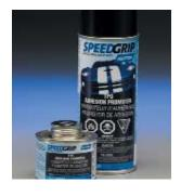
SpeedGrip TPO Adhesion Promoter is available in both aerosol and brush top. To test for TPO plastic, lightly sand an inconspicuous spot on the plastic to be repaired with a 36 grit NorZon Speed-Lok TR disc. If the area melts and/or smears, then it is TPO plastic. If it sands cleanly, then it is not TPO.
